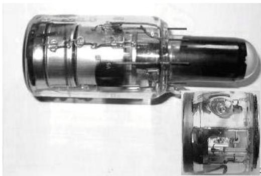
*The 1P25 converter tube with a British Tabby tube inset. To the right the viewing screen on the Tabby is flat, but the 1P25 has a narrow domed screen, which required a special lens to produce a linear image. (1P25 image courtesy Brian Weber, USA.)*
