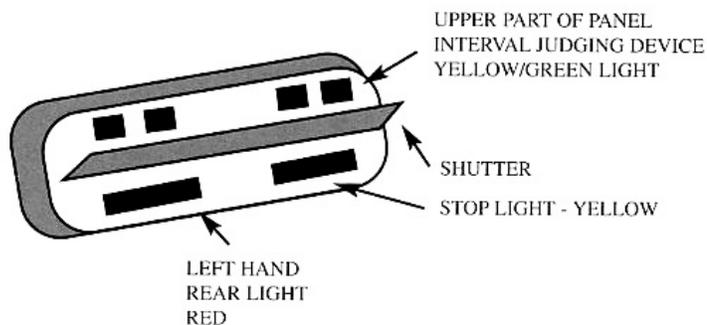
*Rear interval-judging panel and stop light fitted on left-hand rear of vehicle*
