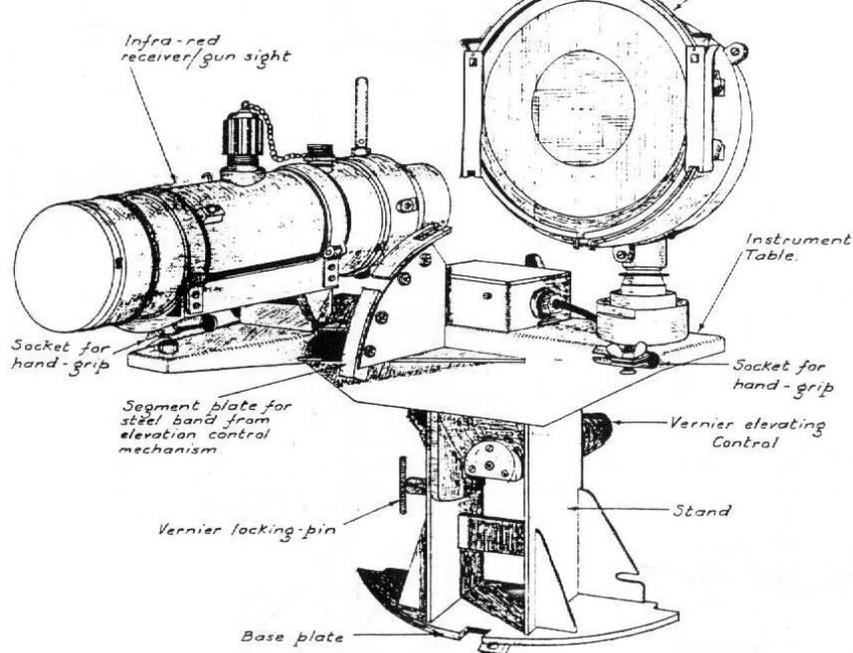
*The Panther tank infra-red set-up, versions of this drawing have been used in a number of books, but this is the original by GSI (Tech) HQ 21 Army Group.*
