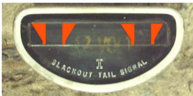
At less than 60 feet from the vehicle in front all four “cats eyes” are distinguishable, beyond 60 feet the closest “cats eyes” appear as one so only two lights are visible. Beyond 180 feet then all the “cats eyes” appear as one light.
