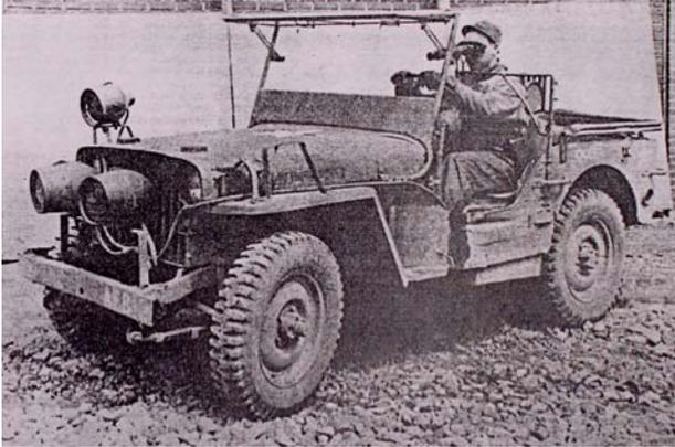
*Type B viewer, and three 450 watt infra-red spotlights. The generator to power the spotlight was carried in the back of the Jeep.*
