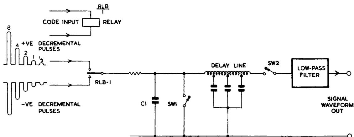
Fig. 4 - Basic de-coding circuit
