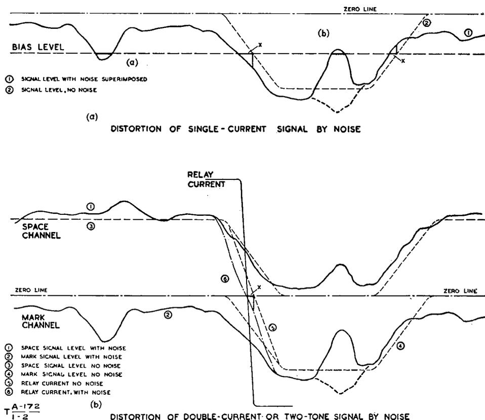
Fig. 2—Distortion due to noise
