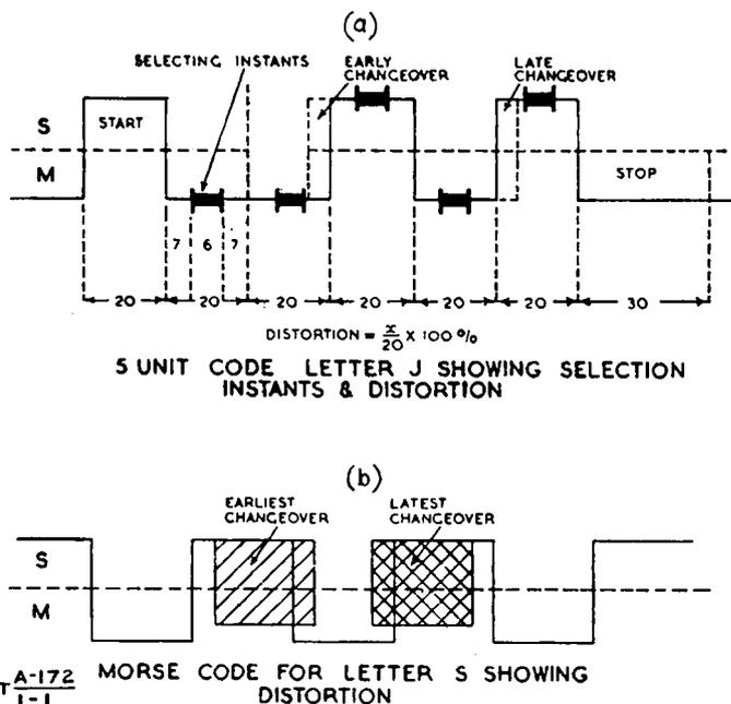
**Fig. 1—Comparison of teleprinter and morse code signals**
