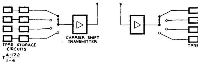
Fig. 4—Simple time division multi-channel system
