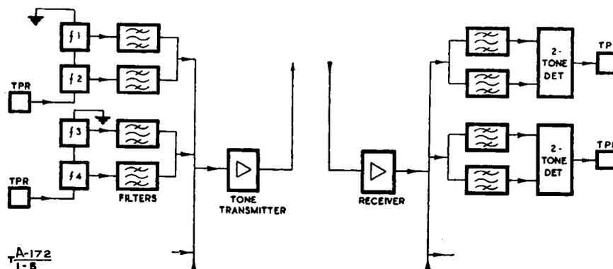
Fig. 5—Simple frequency division multi-channel system
